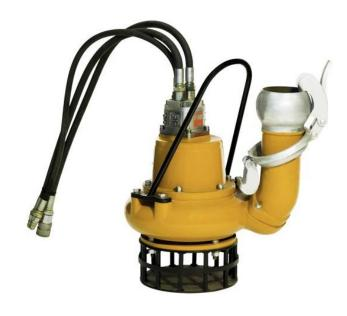
Discharge Size 100 mm Solids Size 50 mm Weight 59 kg 600 mm Height Width (max.) 470 mm Max. Head 35 m Max. Output 50 l/s H.P. Nominal 10 kw Hvdraulic Flow 30 l/min Hydraulic Pressure 205 bar Power Pack 20 Series
