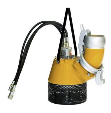
**High Head** Discharge Size 75 mm Solids Size 10 mm Weight 55 kg Height 710 mm Width (max.) 560 mm Max. Head 76 m Max. Output 17 l/s H.P. Nominal 10 kw Hydraulic Flow 30 l/min Hydraulic Pressure 205 bar Power Pack 20 Series
