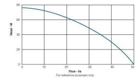
**High Head** Discharge Size 100 mm Solids Size 10 mm Weight 135 kg Height 775 mm Width (max.) 660 mm Max. Head 76 m Max. Output 50 l/s H.P. Nominal 20 kw Hydraulic Flow 63 l/min Hydraulic Pressure 205 bar Power Pack 30 Series
