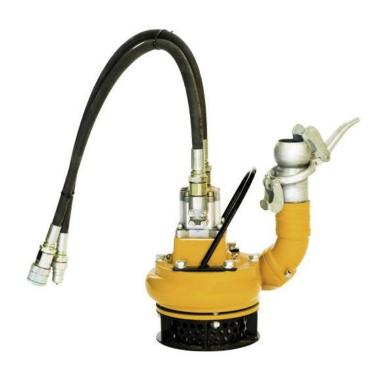
Discharge Size 50 mm Solids Size 10 mm Weight 21 kg Height 300 mm Width (max.) 320 mm Max. Head 28 m Max. Output 50 l/s H.P. Nominal 4.5 kw Hvdraulic Flow 30 l/min Hydraulic Pressure 136 bar Power Pack 10 Series
