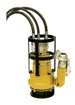
Discharge Size 50 mm Solids Size 10 mm Weight 38 kg Height 445 mm Width (max.) 320 mm Max. Head 49 m Max. Output 17 l/s H.P. Nominal 4.5 kw Hvdraulic Flow 30 l/min Hydraulic Pressure 136 bar Power Pack 10 Series
